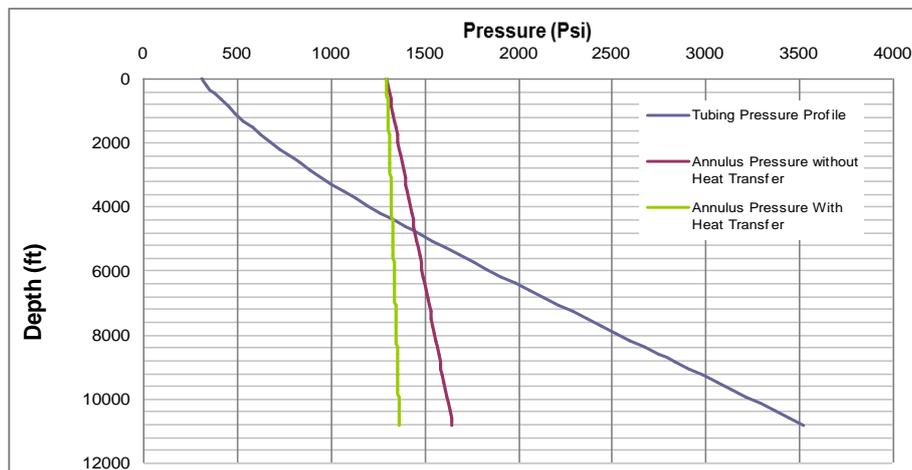
Figure 2. Comparison of Pressure profile in the annulus with and without heat transfer
