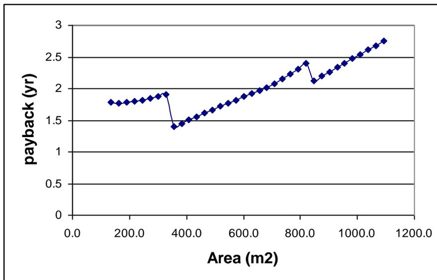
Figure 10. The Correlation between the Payback and the Total Heat Recovery Area
