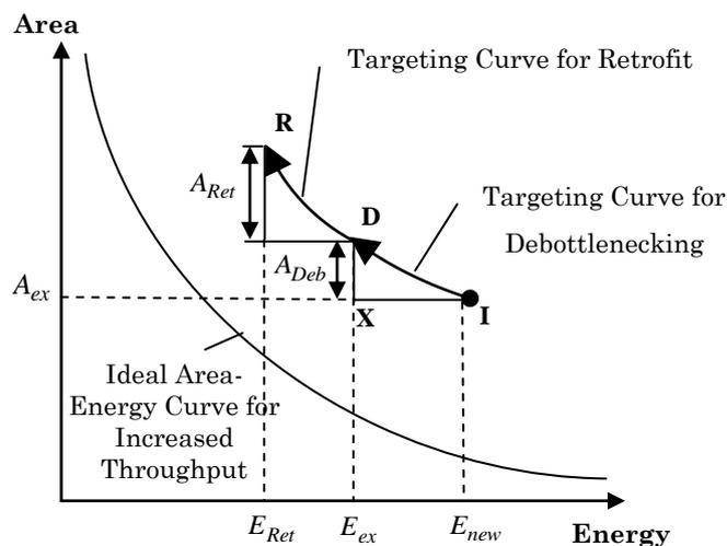
Figure 4. Simultaneous Area, Energy and Throughput Targeting
