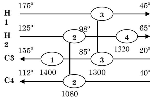
Figure 5. The Existing Heat Exchanger Network
