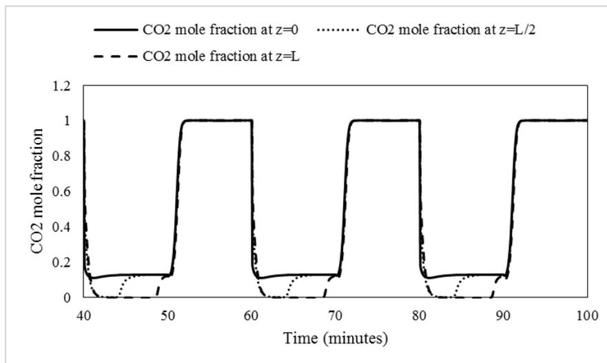
Figure.10. Profile of CO<sub>2</sub> mole fraction at  $z=0$ ,  $z=L/2$ , and  $z=L$  versus time for three last cycles out of 5.
