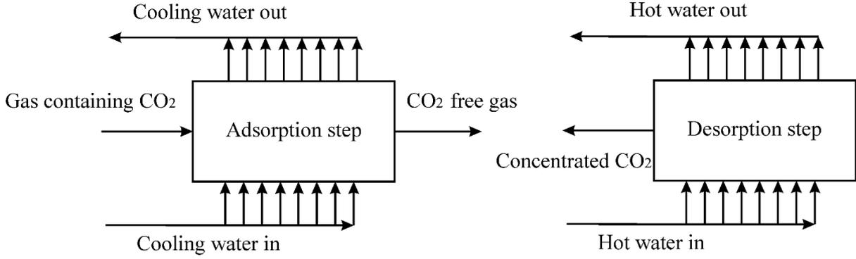
Figure.2. schematic representation of adsorption and desorption step
