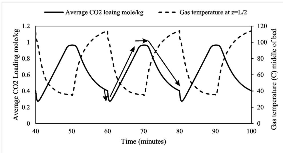
Figure.9. Profile of average CO<sub>2</sub> loading and gas temperature at  $z=L/2$  versus time for three last cycles out of 5.
