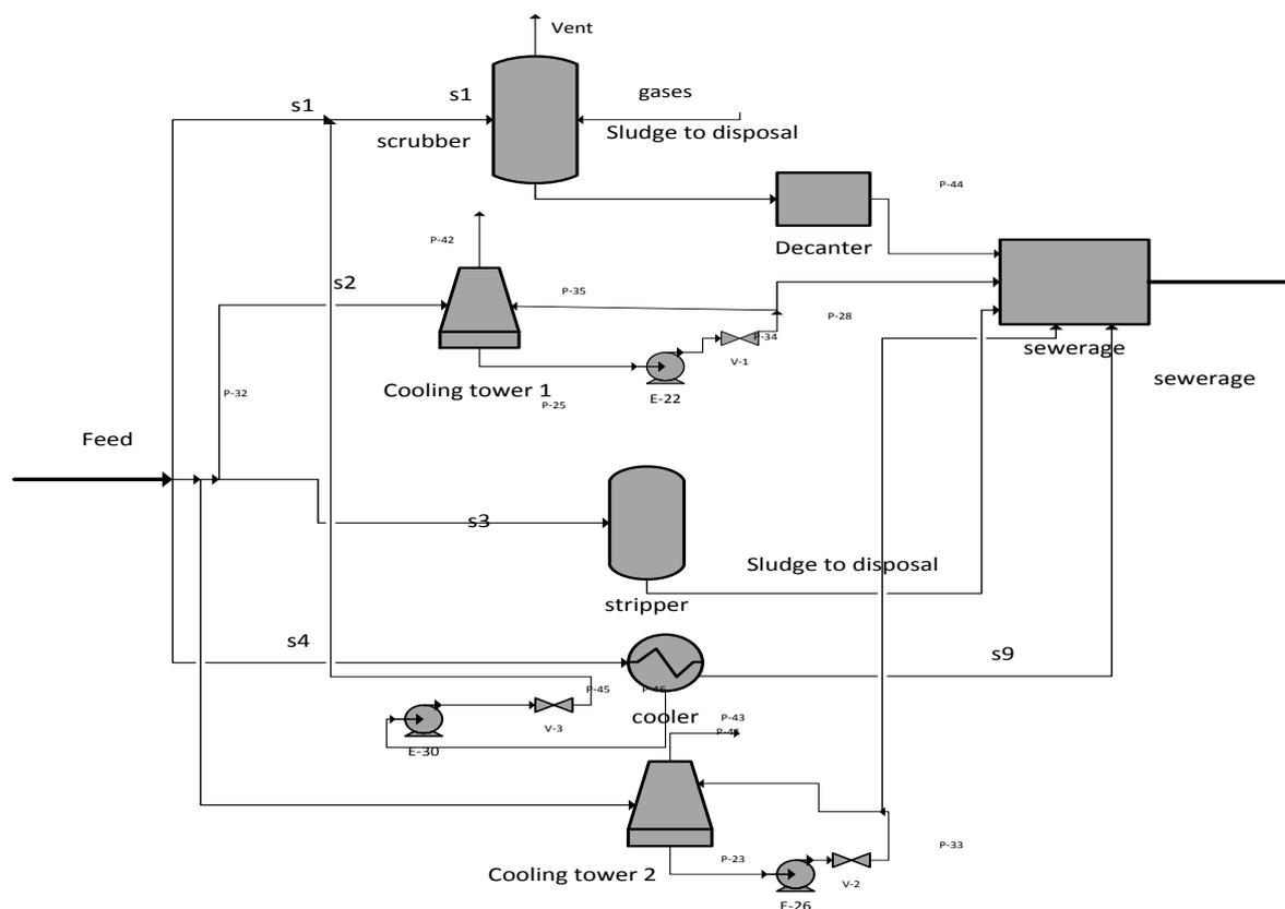
Figure 1. Water Network of selected Gas Refinery
