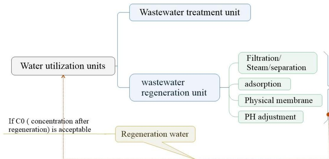
Figure 3. Schematic of the regeneration unit
