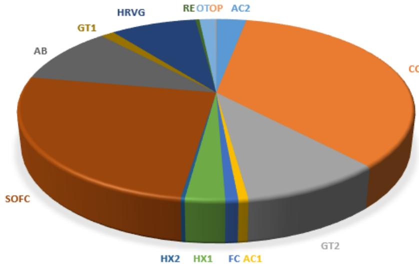
Figure 3. Exergy destruction distribution in SOFC-GT-ORC combined cycle
