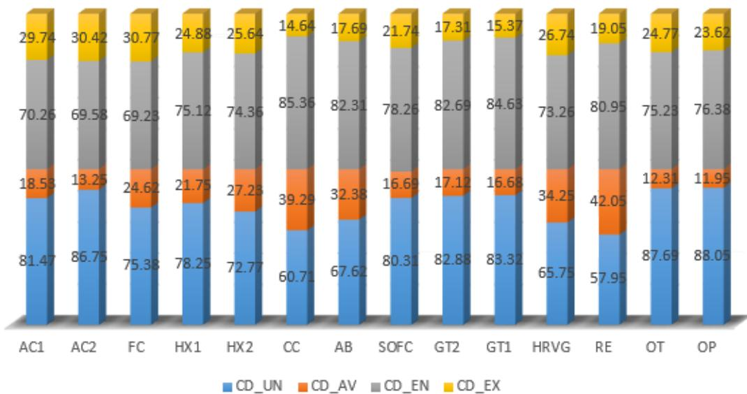
Figure 5. The percent of avoidable/unavoidable and exogenous/endogenous exergy destruction cost rate of SOFC-GT-ORC components
