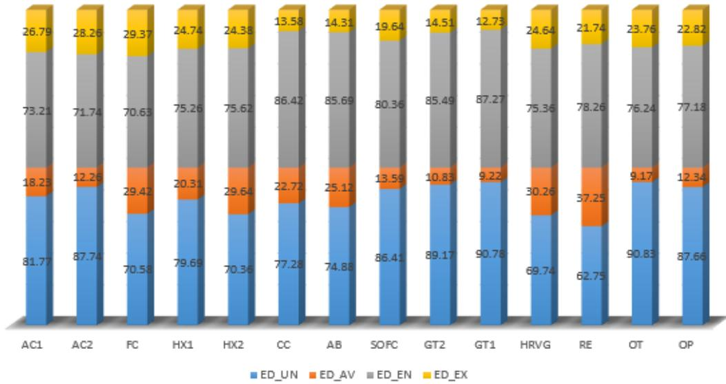
Figure 4. Distribution of avoidable/unavoidable and exogenous/endogenous Exergy Destruction of SOFC-GT-ORC components
