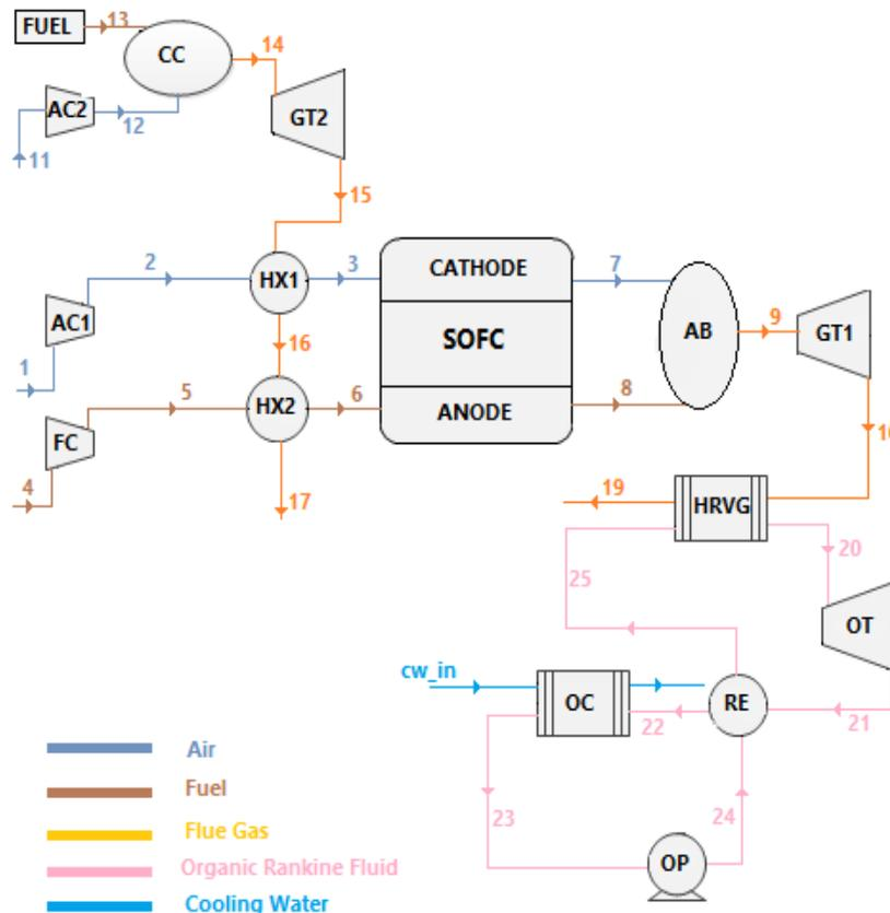
Figure 1. Schematic of the proposed hybrid system Schematic must be capital
