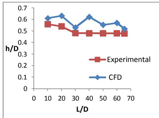
**Fig. 10.** The mean liquid height as a function of pipe inlet and slope onset to slugging. ( $U_{SL} = 0.14(m/s)$  and  $U_{SG} = 2.4(m/s), \theta = 0.0$ )
