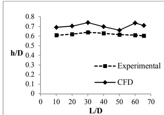
Fig. 12. The mean liquid height as a function of pipe inlet and slope onset to slugging. ( $U_{SL} = 0.53(m/s)$  and  $U_{SG} = 2.4(m/s), \theta = -0.8^\circ$ )
