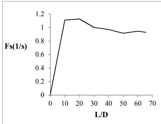
Fig. 16. Examining slug frequency along the horizontal pipeline according to Zabaraz correlation
