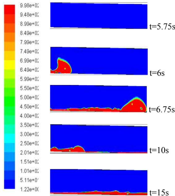
Fig. 6. The changes of slug length by passing time in pipe with  $\theta = -0.8^\circ$
