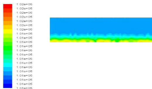
Fig. 18. The contours of absolute pressure in horizontal pipe in 10s
