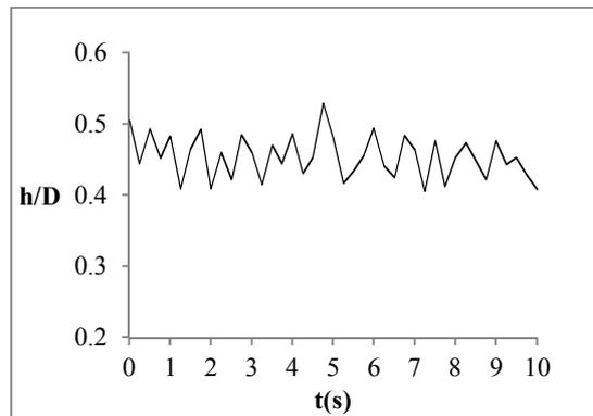
Fig. 13. The effect of slope on the liquid hold up in  $L/D = 30$  and  $\theta = 0.0$
