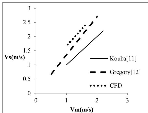
Fig. 17. The correlation between slug translational velocity and fluid mixture velocity.
