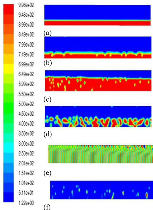
**Fig. 3.** Horizontal two phase flow regimes. Contours of mixture density for water-air (a) stratified flow (b) wavy flow (c) plug flow (d) slug flow (e) bubble flow (f) spray flow.
