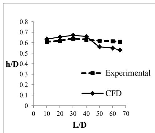
**Fig. 11.** The mean liquid height as a function of pipe inlet and slope onset to slugging. ( $U_{SL} = 0.53(m/s)$  and  $U_{SG} = 2.4(m/s), \theta = -0.5^\circ$ )
