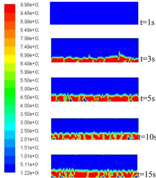
Fig. 5. The changes of slug length by passing time in the horizontal pipe
