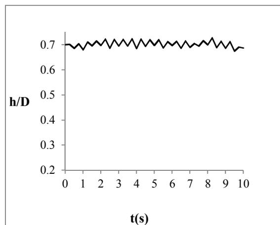
Fig. 15. The effect of slope on the liquid hold up in  $L/D = 30$  and  $\theta = -0.8^\circ$
