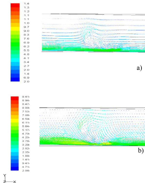
Fig. 21. Internal structure of a slug velocity field a)  $\theta = 0.5^\circ$  b)  $\theta = -0.8^\circ$
