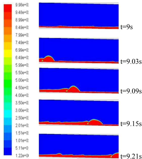
Fig. 7. Slug formation with  $U_{SG} = 2/4$  (m/s) and  $U_{SL} = 0.59$  (m/s)  $\theta = -0.5^\circ$
