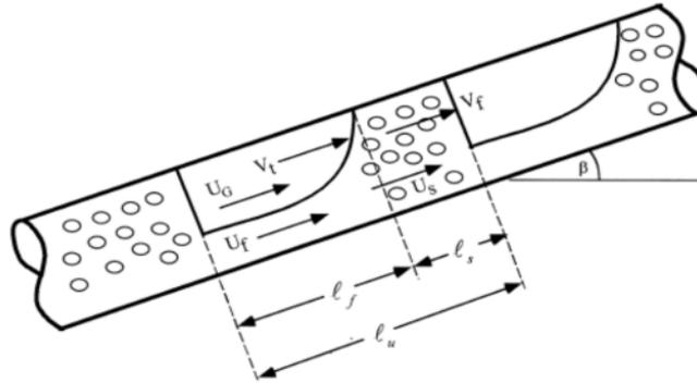
Fig. 2. Slug flow geometry
