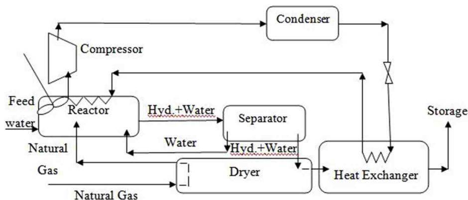
Fig. 2. Schematic NGH Production Process
