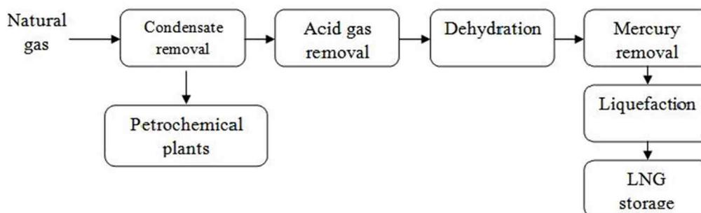
Fig. 1. A typical LNG chain
