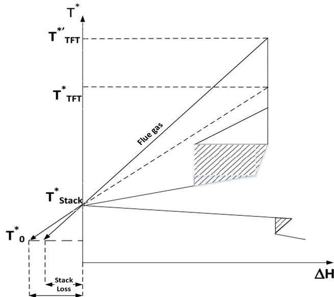
Figure 15. Effect of higher duct burner outlet temperature in the HRSG performance
