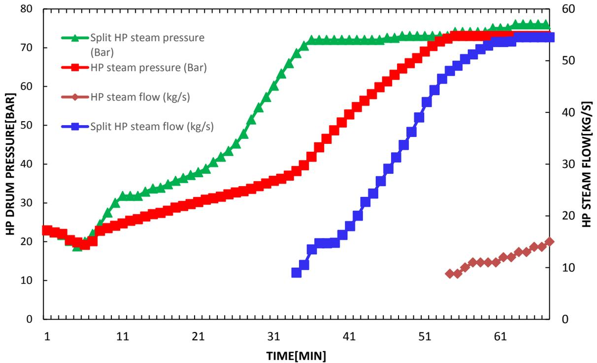
Figure 18. Effect of splitting on pressure and mass flow rate of HP stream
