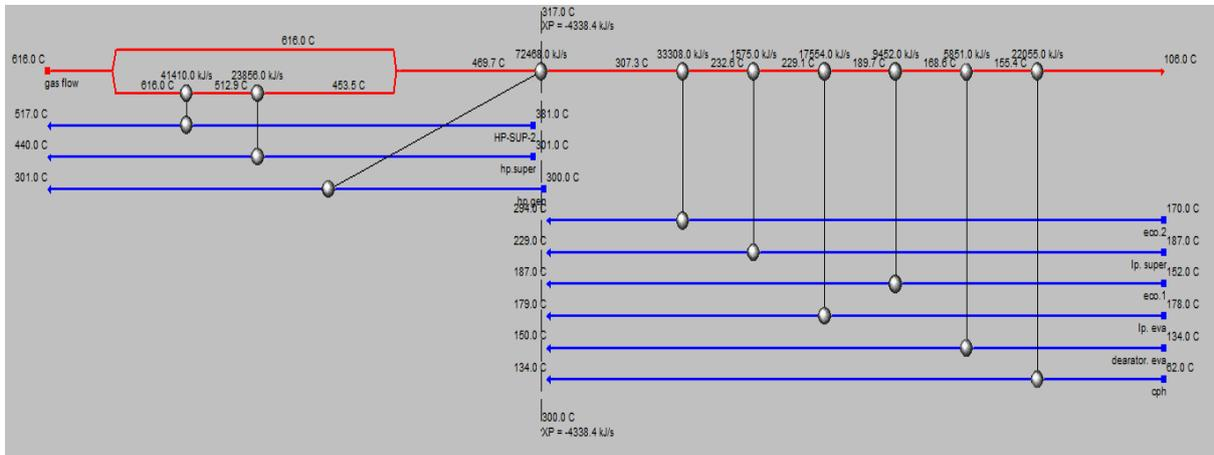
Figure 12. Heat exchanger network design after splitting
