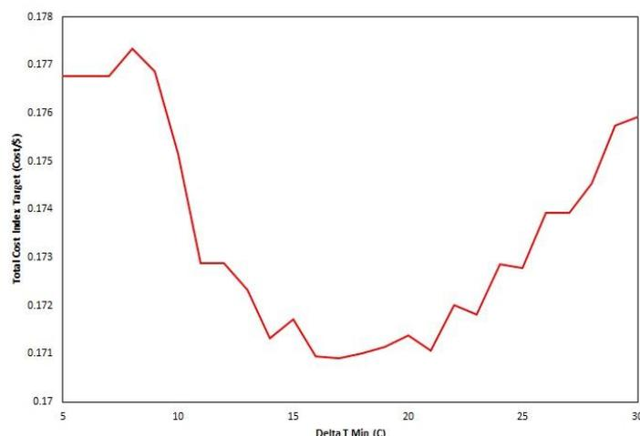
Figure 7. Variation of total cost of HRSG with minimum temperature difference
