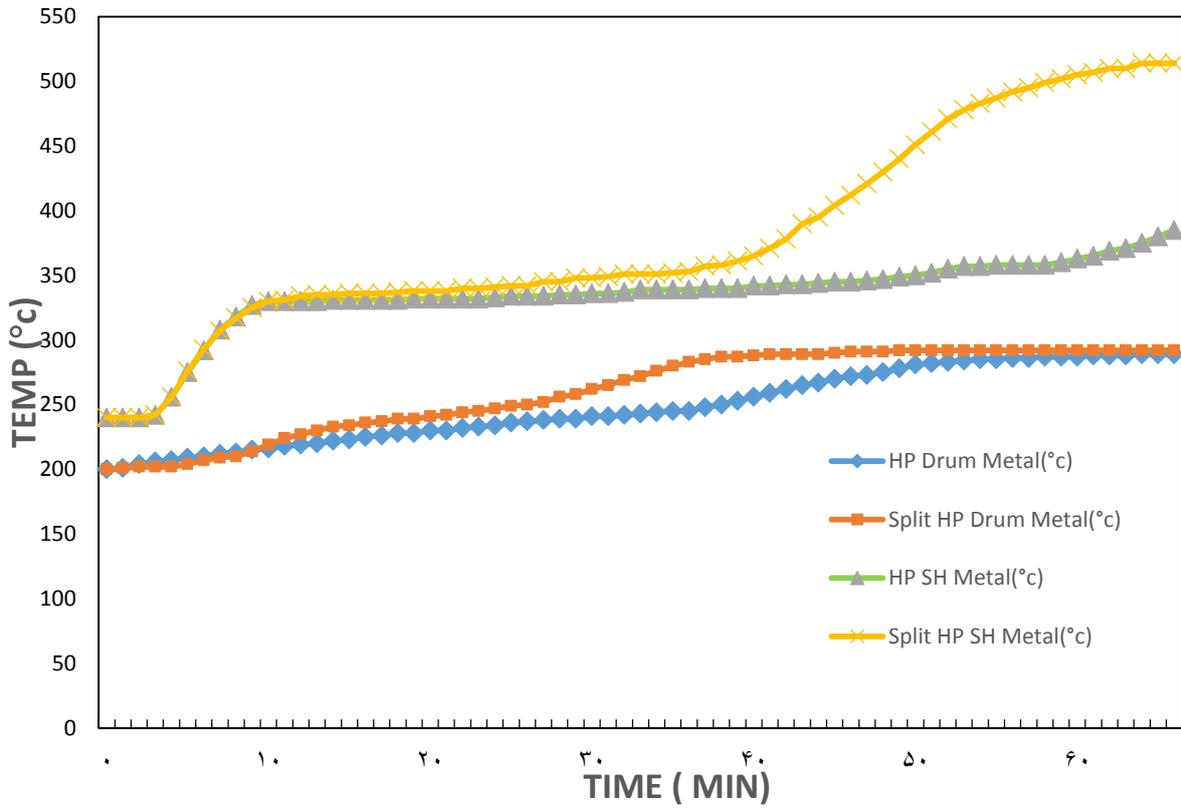
Figure 17. Effect of splitting process on temperature of evaporator and super heater wall
