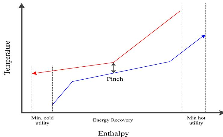
Figure 3. Composite curve for a sample process
