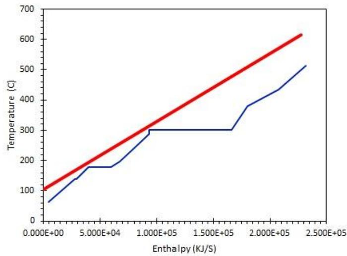
Figure 13. Composite curve of HRSG after splitting
