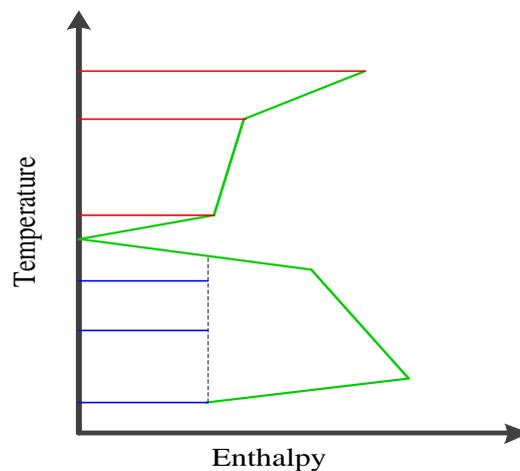
Figure 4. Grand composite curve for a sample process
