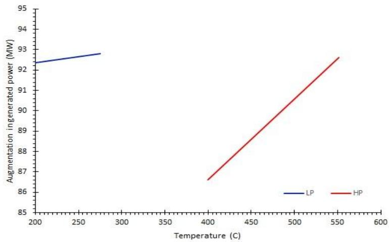
Figure 16. Effect of HP and LP steam temperature on generated power by steam turbine
