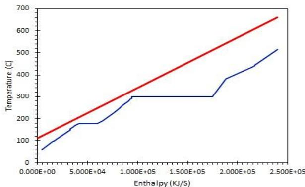
Figure 10. Composite curve for HRSG during summer
