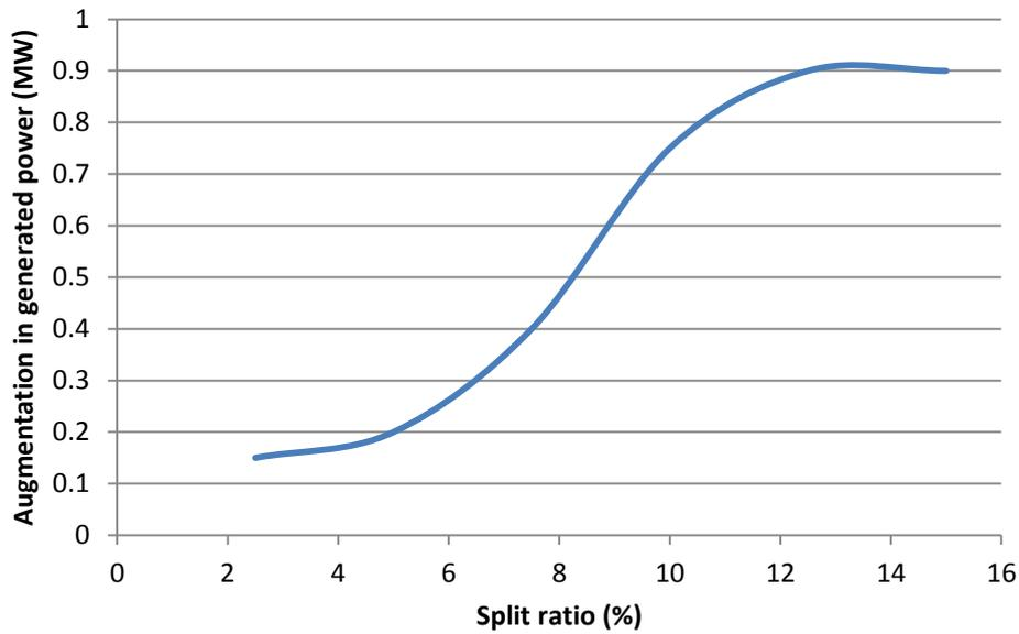
Figure 20. The effect of split ratio on generated power by steam turbine
