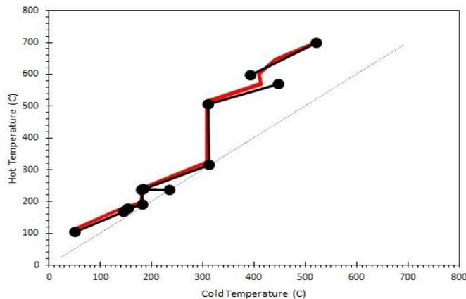
Figure 9. Driving force plot of the HRSG in base case condition
