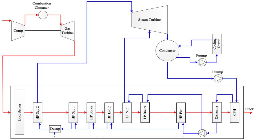
Figure 1. Schematic diagram of Damavand power plant
