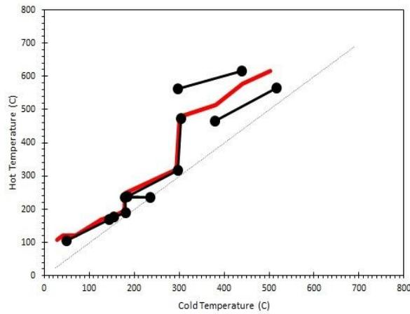
Figure 11. Driving force plot of the HRSG during summer
