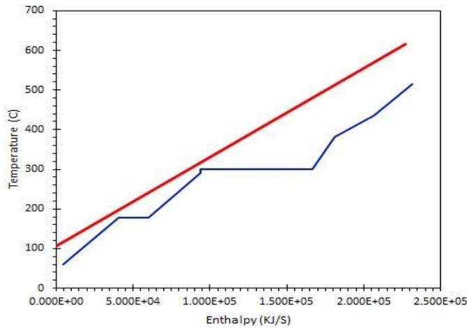
Figure 8. Composite curve for HRSG in base case condition
