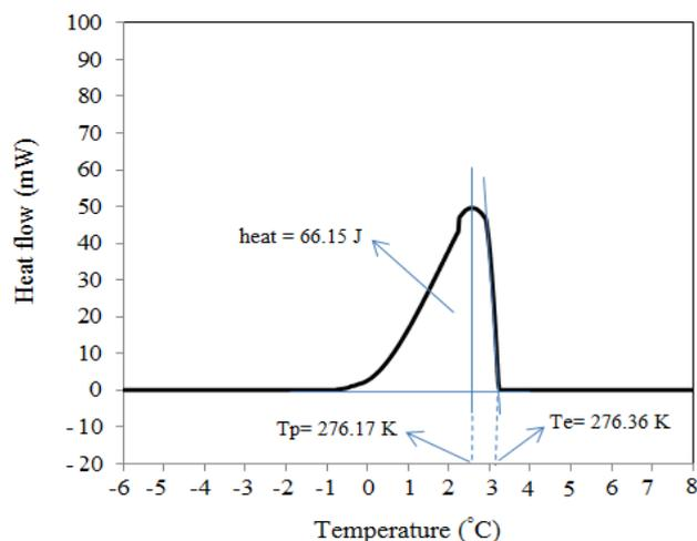
Figure 3. DSC curve of THF hydrate formation. ( $T_p$ : temperature of peak,  $T_e$ : phase change temperature)
