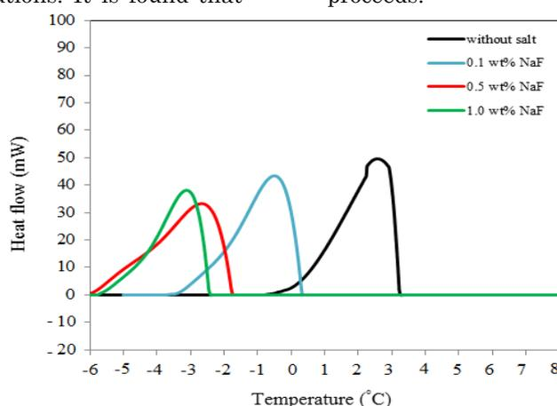
Figure 5. DSC curve of THF hydrate formation at various NaF concentrations.
