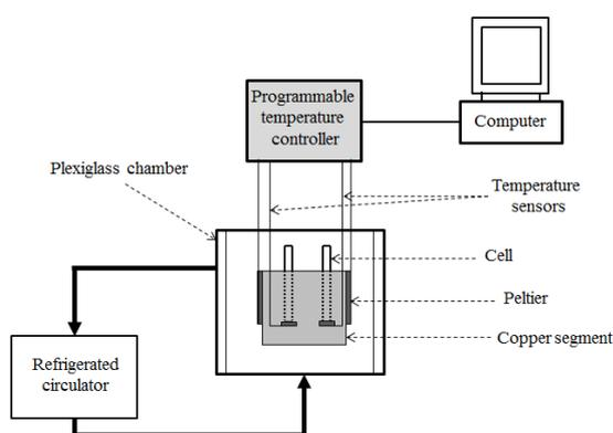
**Figure 1.** Schematic diagram of the experimental apparatus of DSC.
