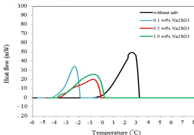
Figure 6. DSC curve of THF hydrate formation at various Na<sub>2</sub>SO<sub>3</sub> concentrations.
