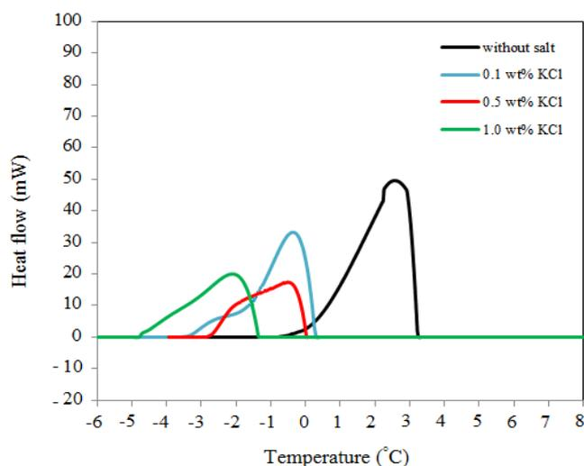
Figure 7. DSC curve of THF hydrate formation at various KCl concentrations.
