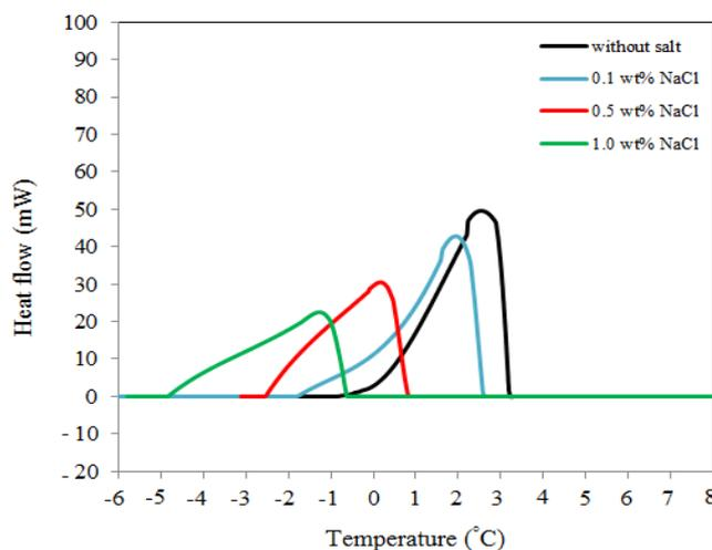
Figure 4. DSC curve of THF hydrate formation at various NaCl concentrations.
