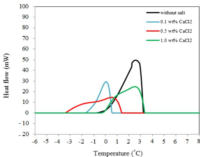
Figure 8. DSC curve of THF hydrate formation at various  $\text{CaCl}_2$  concentrations.
