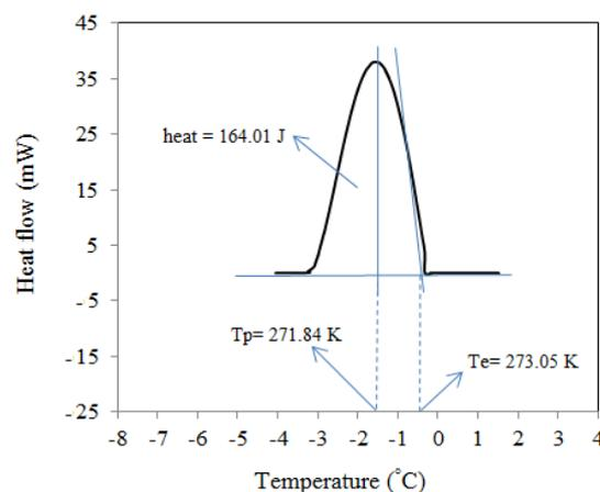
**Figure 2.** DSC freezing curve of ice. (Tp: temperature of peak, Te: phase change temperature)
