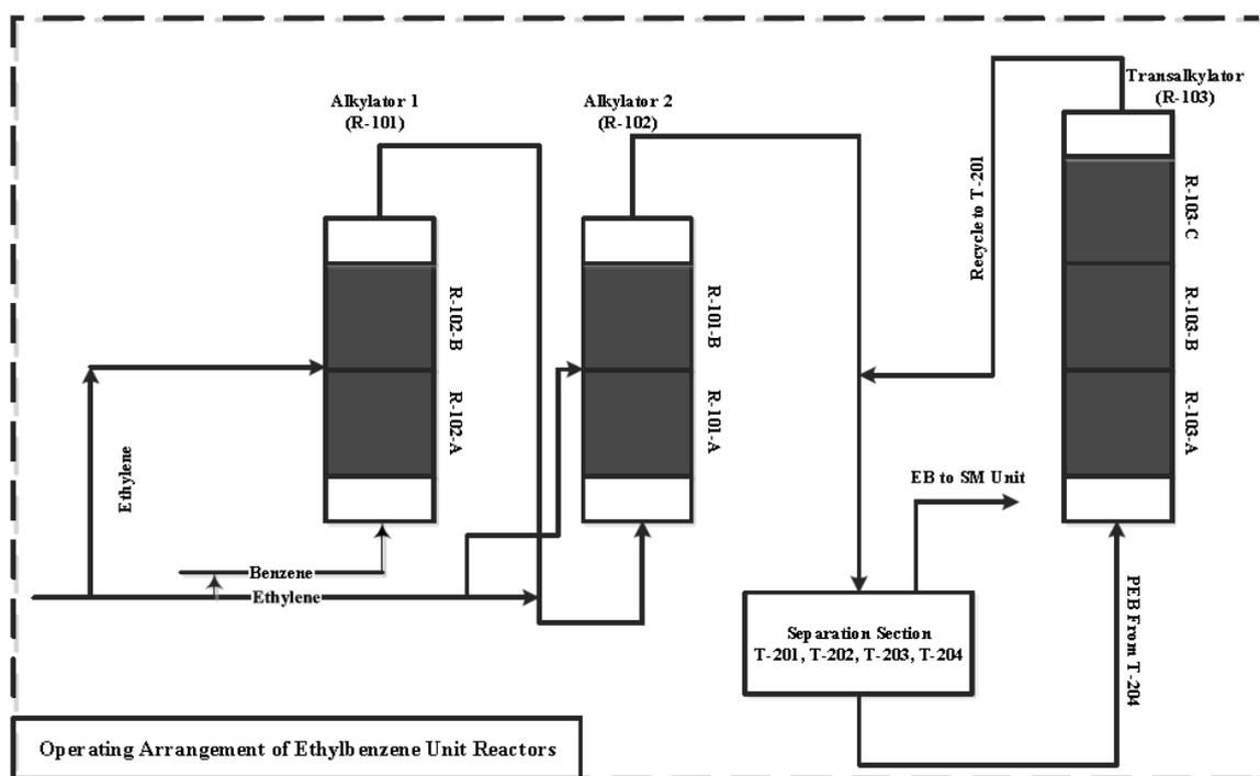
Figure 4. BFD of conventional reactor arrangement of EB unit
