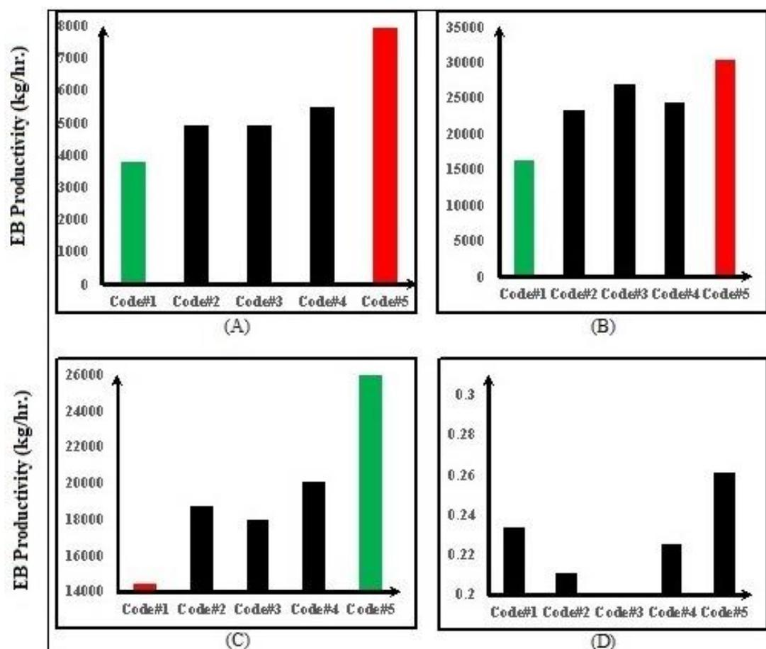
Figure 6. EB Productivity (kg/hr) comparison of various parameters between several arrangement scenarios; A: Ethylene consumption; B: Benzene consumption; C: Ethylbenzene production; D: Ratio of ethylene to benzene
