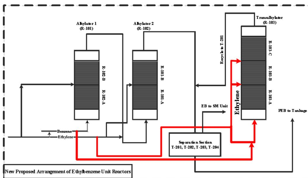
Figure 5. BFD of reactor arrangement for scenario 2 of EB unit
