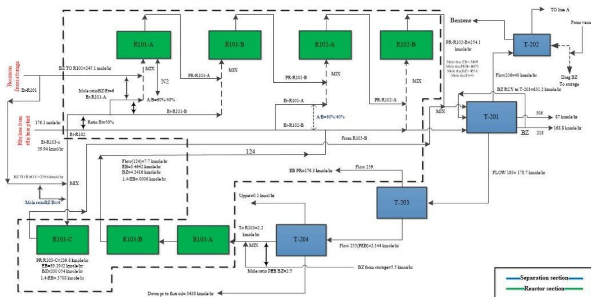
Figure 1. Block flow diagram of ethylbenzene unit
