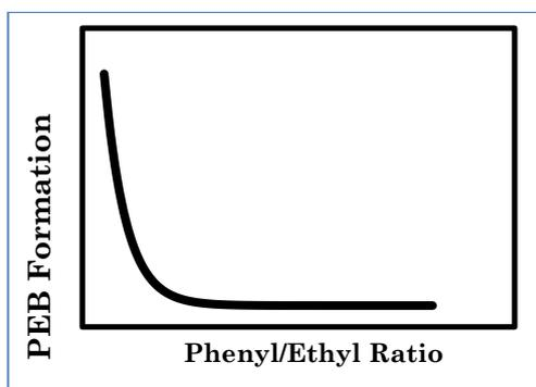
Figure 2. Distribution of PEB at various Phenyl/Ethyl Ratio [Operating Manual of EB Unit, UOP, 1991]
