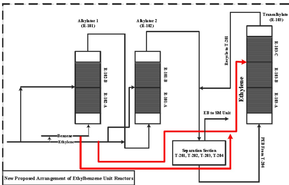
Figure 4. BFD of reactor arrangement for scenario 1 of EB unit
