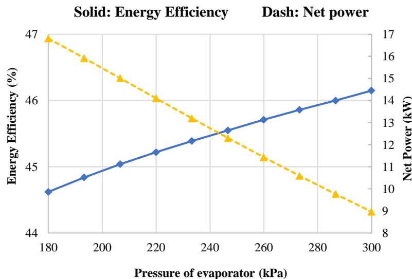
**Figure 5.** Impact of  $P_e$  on the energetic efficiency and net power
