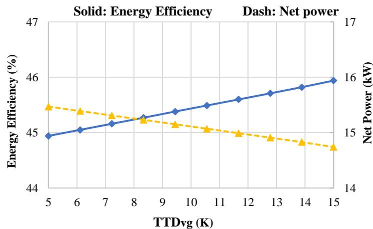
Figure 2. Impact of  $TTD_{v,g}$  on the energetic efficiency and net power
