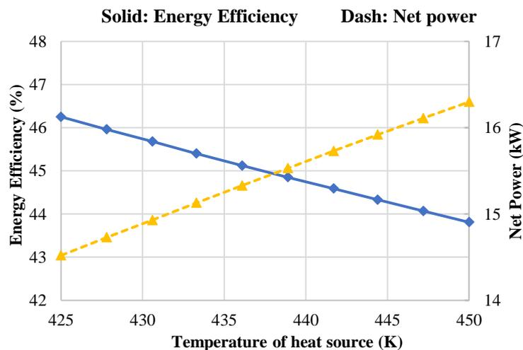
Figure 3. Impact of heat source temperature on the energetic efficiency and net power
