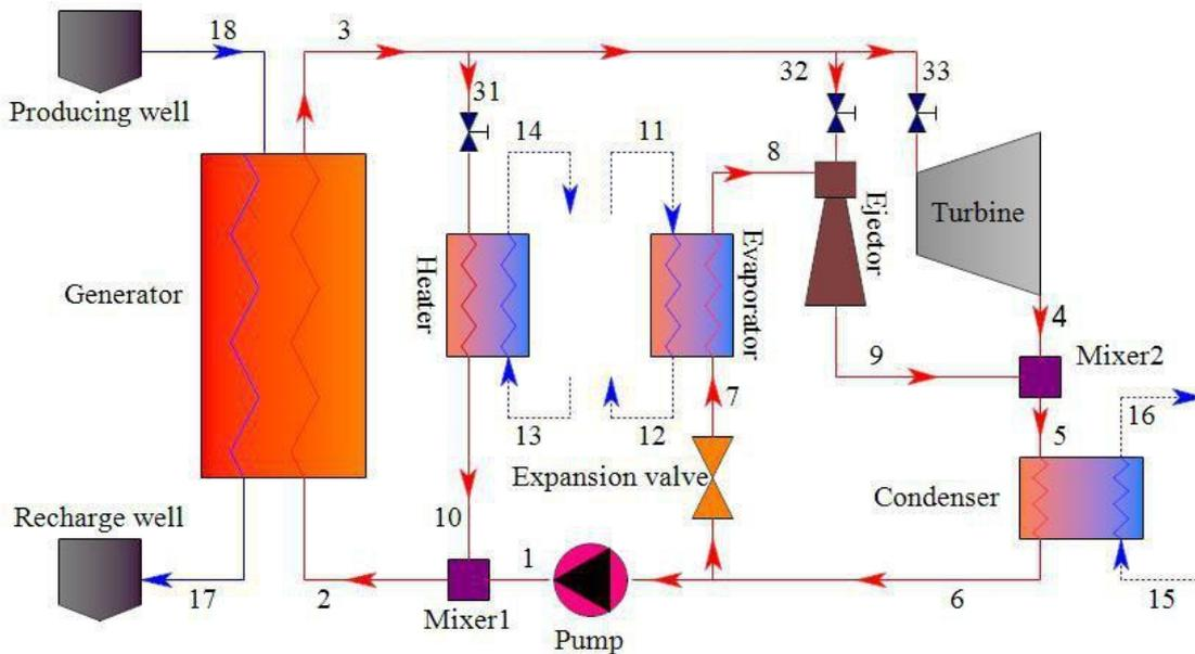
Figure 1. Schematic diagram of the CCHP with geothermal source
