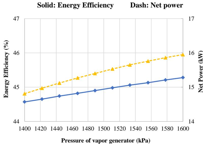
**Figure 4.** Impact of  $P_{vg}$  on the energetic efficiency and net power
