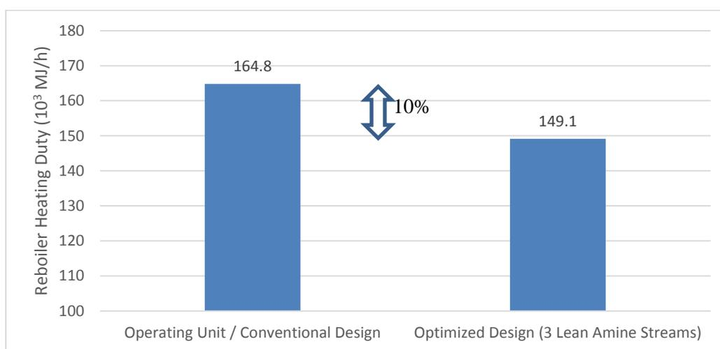
Fig. 7 Comparison of re-boiler heating duty
