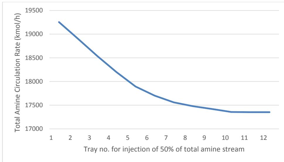
**Fig.3** Application of two lean amine streams into absorber (50% of lean amine solution at 1<sup>st</sup> stage, i.e. top of the contactor, and other 50% at lower stages) and effect on total amine circulation rate
