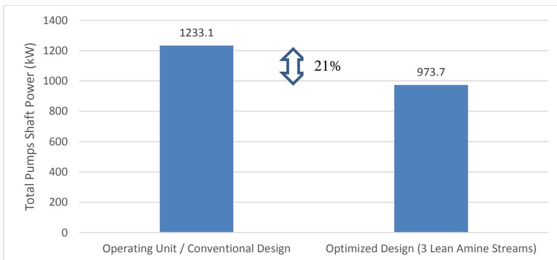
**Fig.5** Comparison of shaft power demand by pumps
