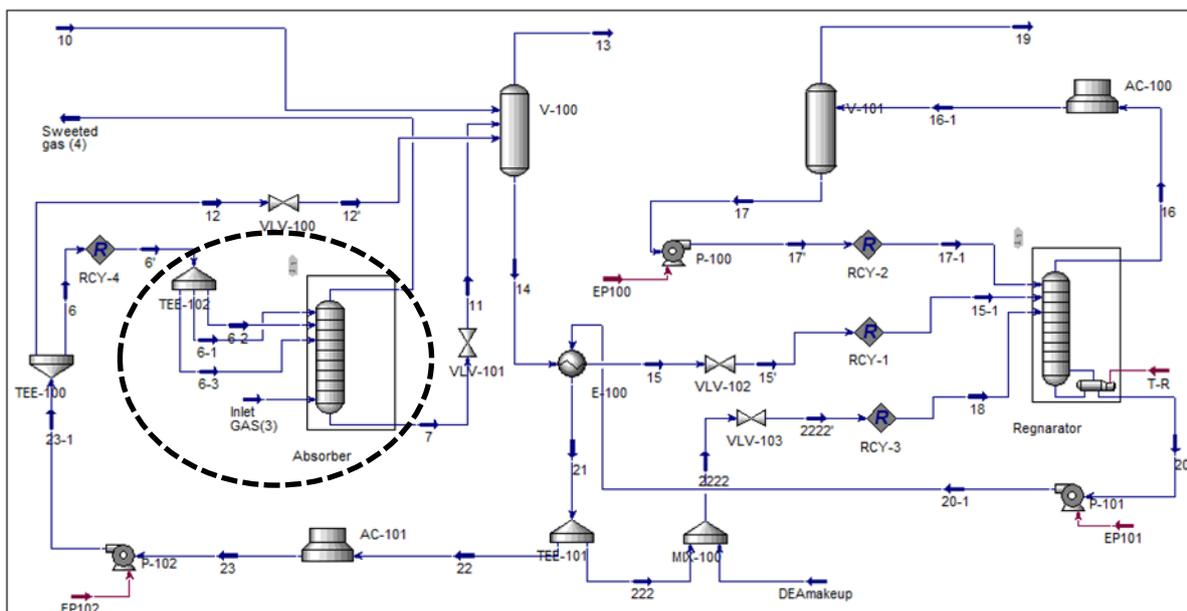
Fig. 2 Application of three lean amine streams to absorber
