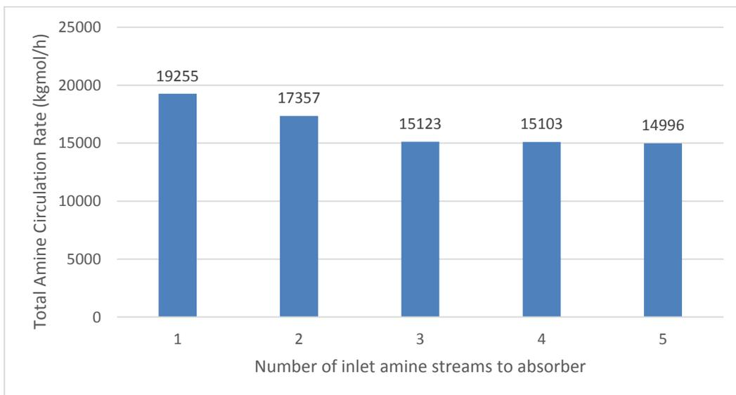
**Fig.4** Changing of the total required amine circulation rate by using multiple lean amine streams.
