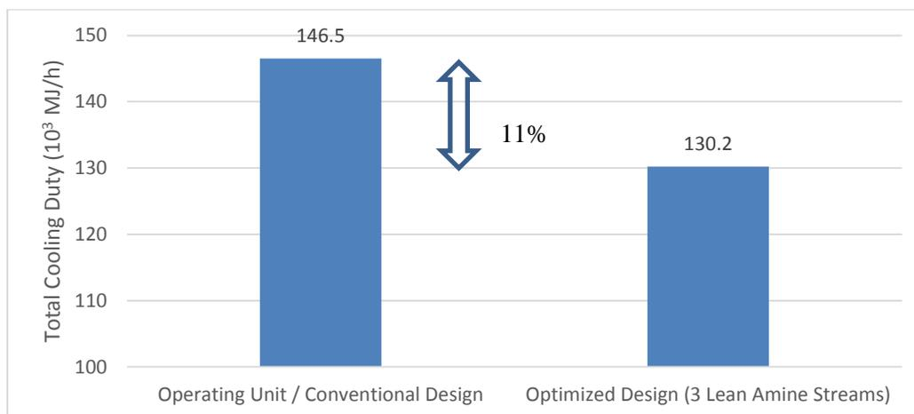
Fig. 6 Comparison of coolers cooling duty
