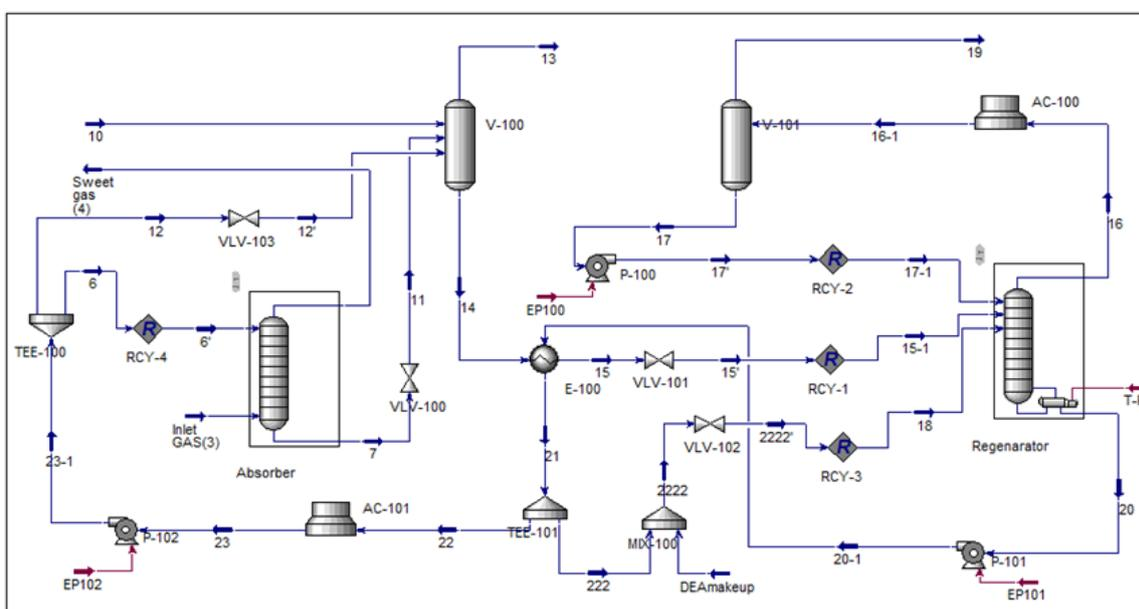
**Fig. 1** Simplified PFD of Amine Unit used in simulation
