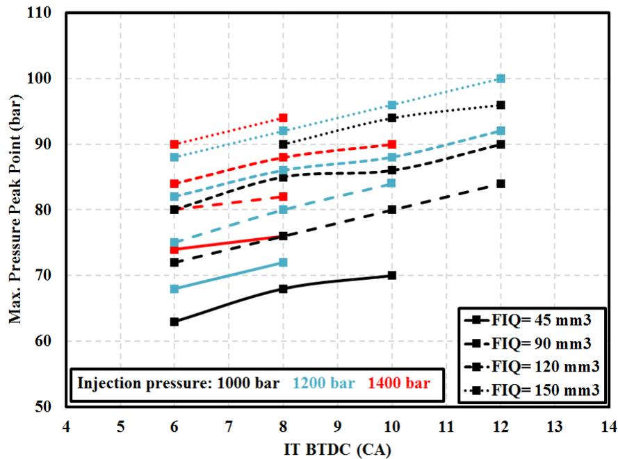
Figure 3. Effects of fuel injection characteristics on the in-cylinder Maximum Pressure Peak point
