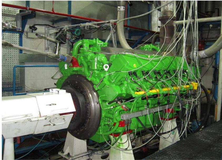
**Figure 1.** D87 Diesel engine in the test room**Table 2.** Measuring Instruments Specification
