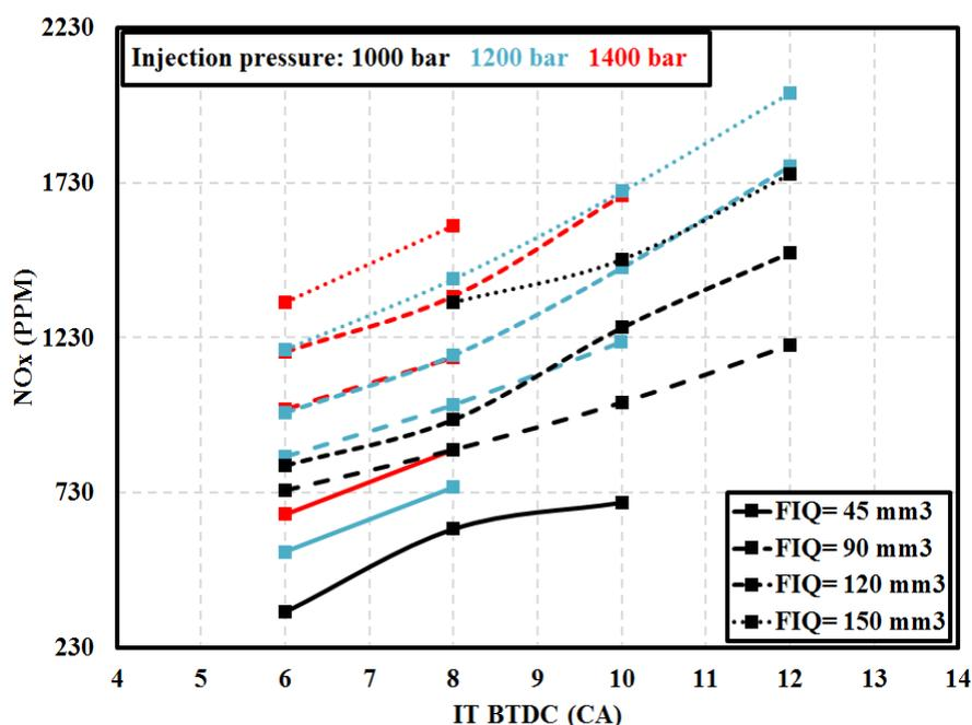
Figure 5. Effects of fuel injection characteristics on NO<sub>x</sub> emissions formation
