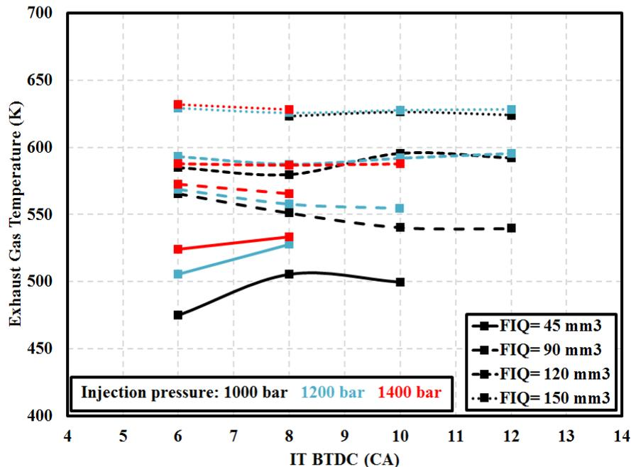
Figure 4. Effects of fuel injection characteristics on the exhaust gas temperature
