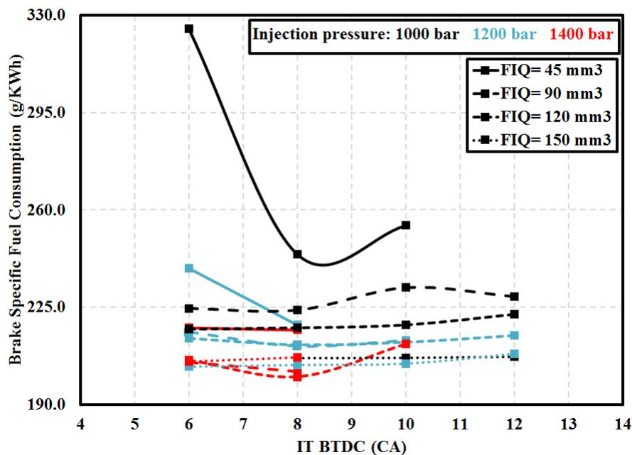
Figure 8. Effects of fuel injection characteristics on BSFC
