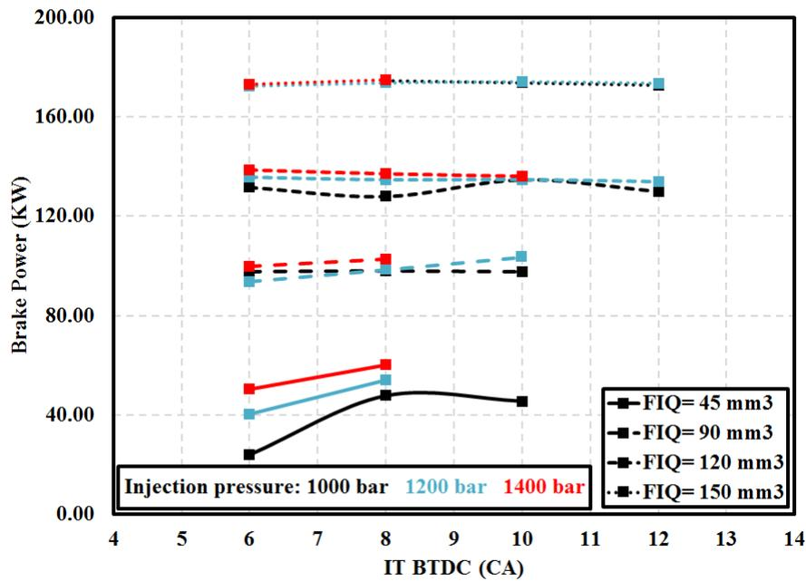
Figure 7. Effects of fuel injection characteristics on brake power
