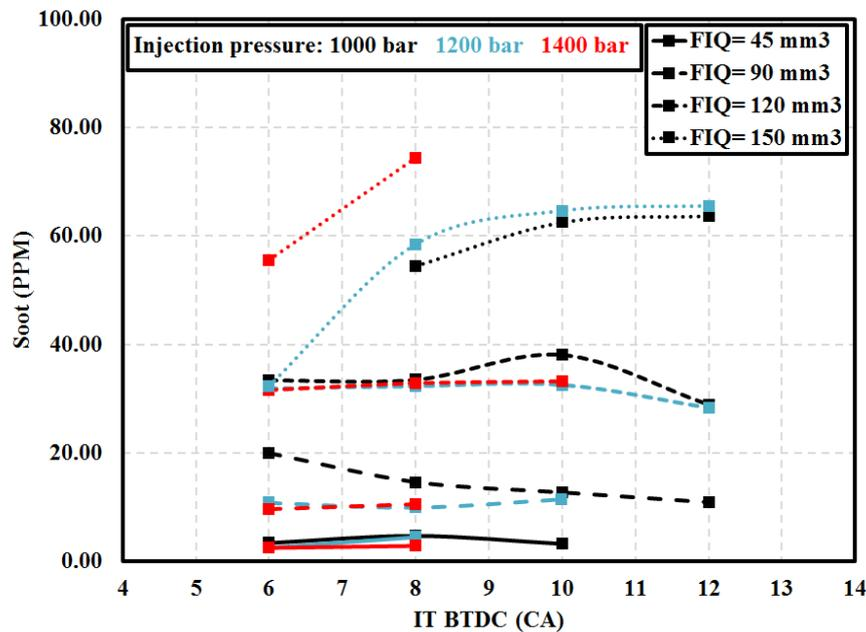
Figure 6. Effects of fuel injection characteristics on soot emission formation
