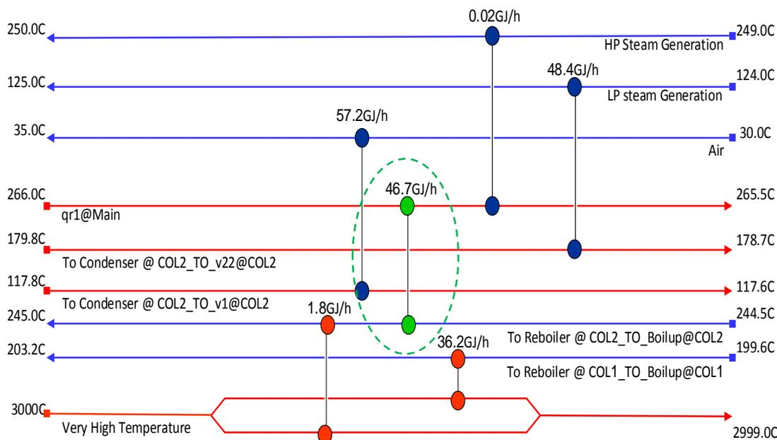
Figure 8. Grid diagram of heat exchanger network for the proposed process after pinch
