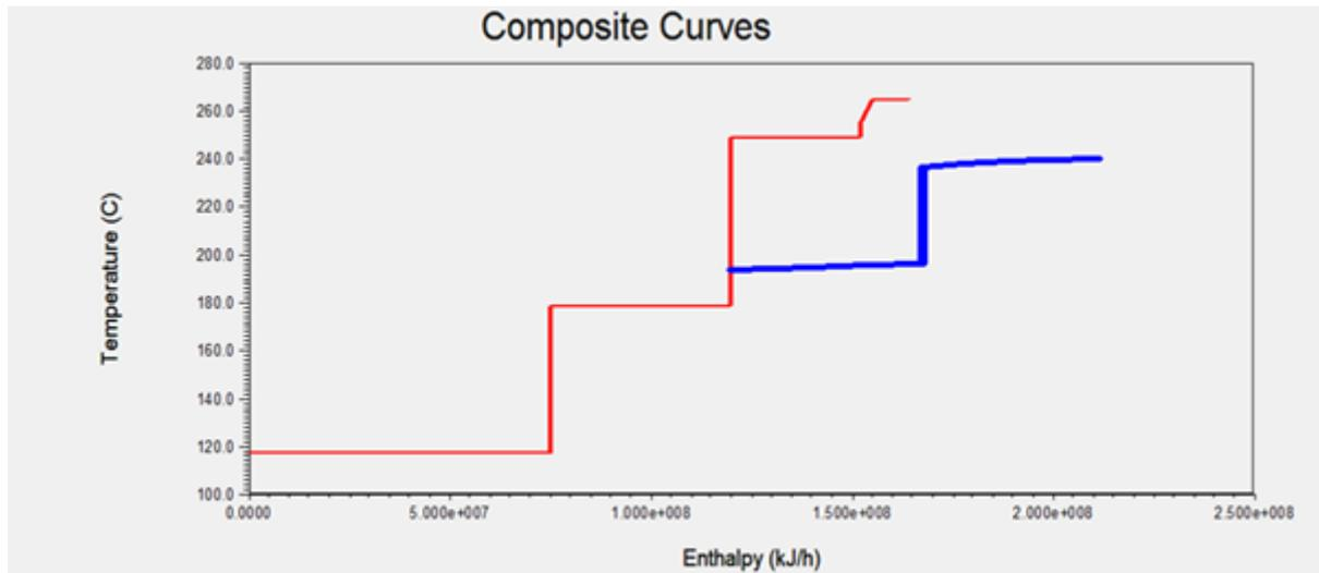
Figure 5. Composite Curve for Conventional Process
