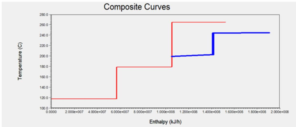
Figure 6. Composite Curve for Proposed Process
