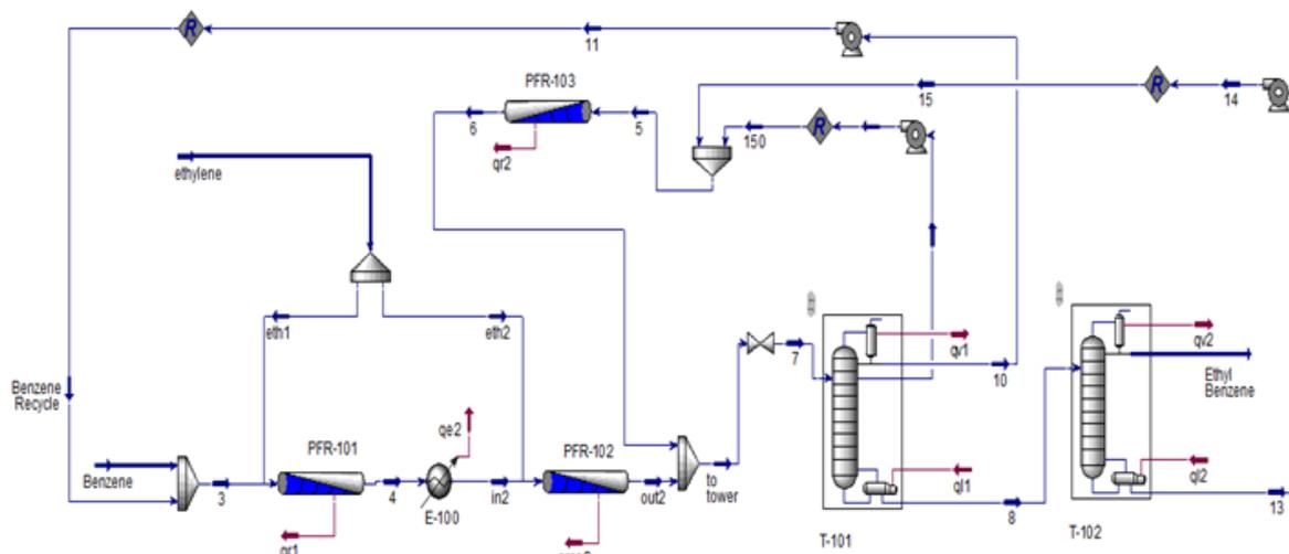
**Figure 1.** Scheme of the conventional process
