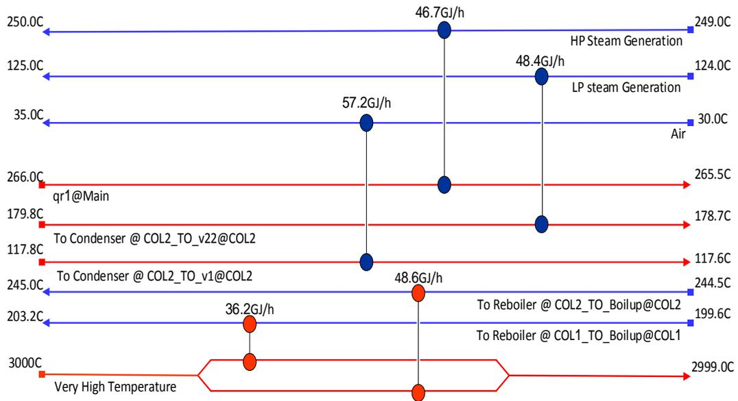
Figure 4. Grid diagram of heat exchanger network for the proposed process
