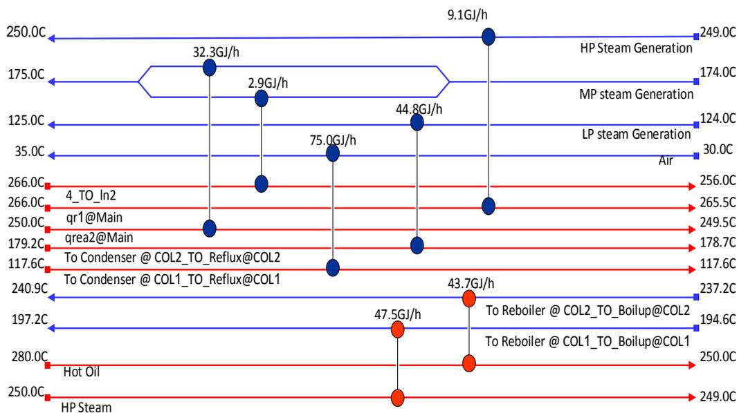
**Figure 3.** Grid diagram of heat exchanger network for conventional process
