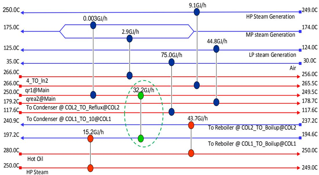
**Figure 7.** Grid diagram of heat exchanger network for the conventional process after pinch
