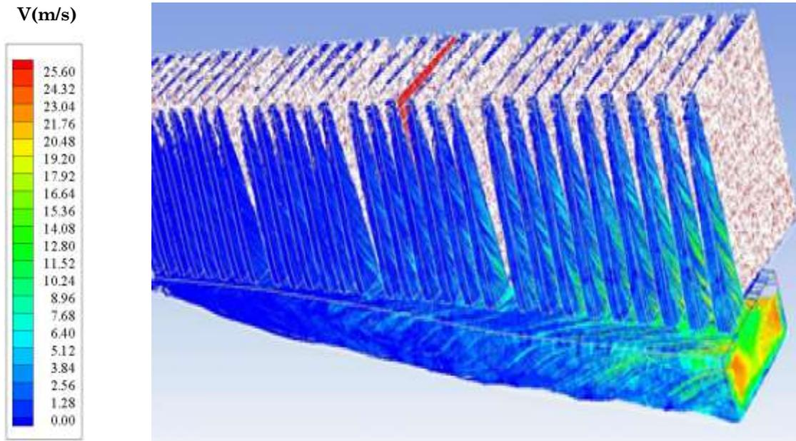
Figure 11. Velocity magnitudes in the entire inertial sand separators and channel
