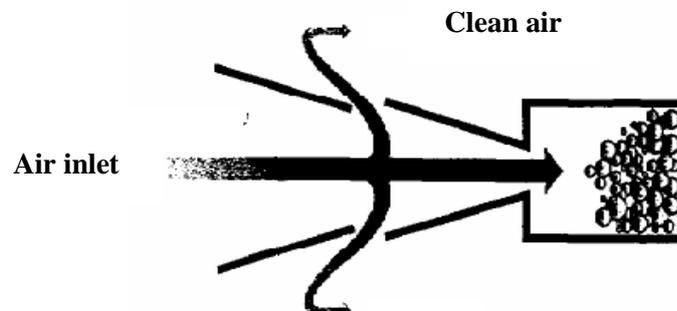
Figure 2. schematic of the air flow in an inertial sand separator
