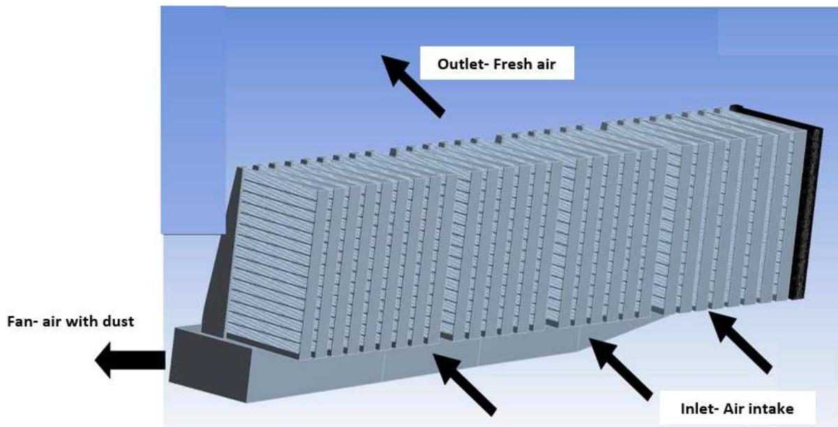
Figure 4. Schematic view of the inertial sand separators
