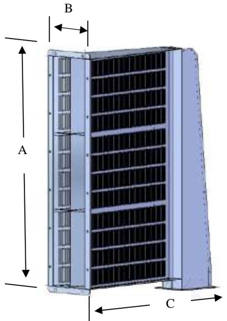
Figure 3. Schematic of an inertial sand separator
