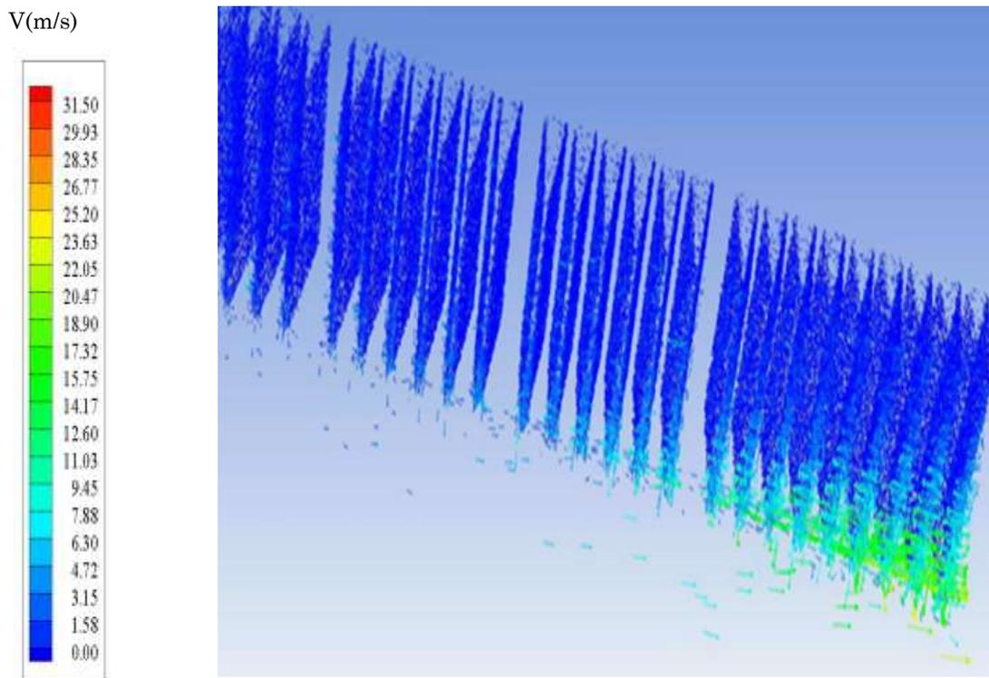
Figure 12. Velocity vectors the entire inertial sand separators and channel
