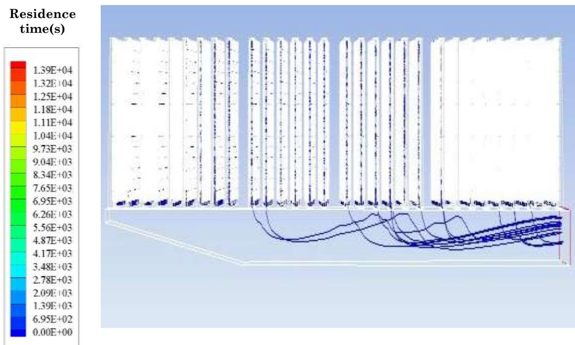
Figure 10. The trajectory of particles in the entire inertial sand separators and channel
