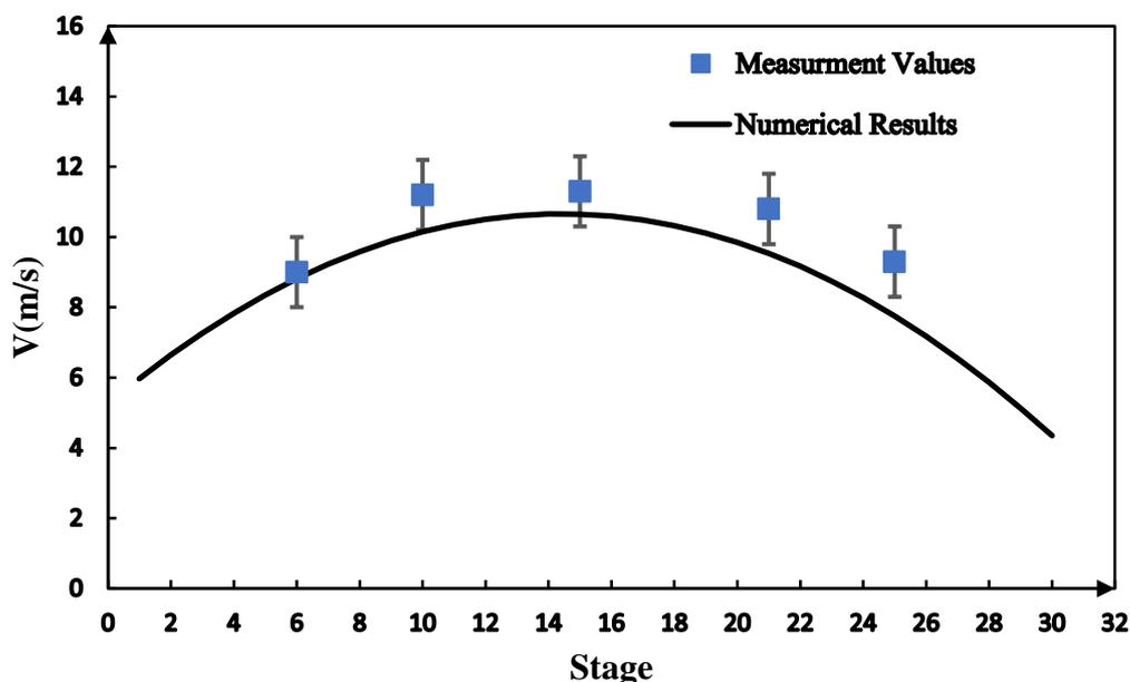
**Figure 8.** Comparison of velocity values obtained from the numerical solution and measurements (*Performance test of Kave combined cycle PP (GT V94.2). (n.d.), n.d.*)
