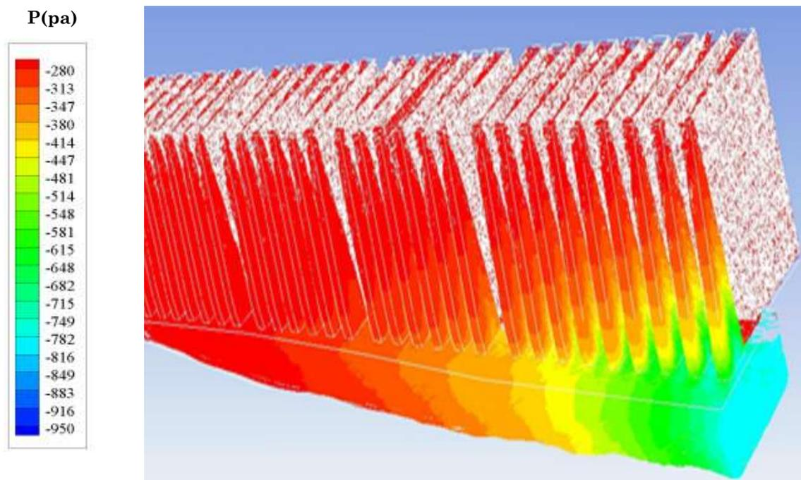
Figure 9. Pressure distribution in the entire inertial sand separators and channel
