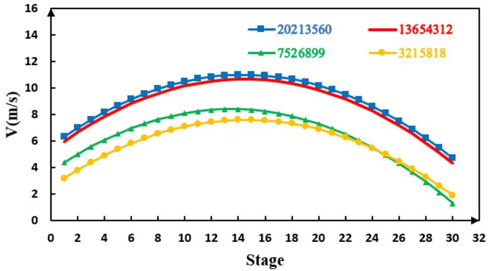
Figure 5. Comparison of velocity values for different meshes
