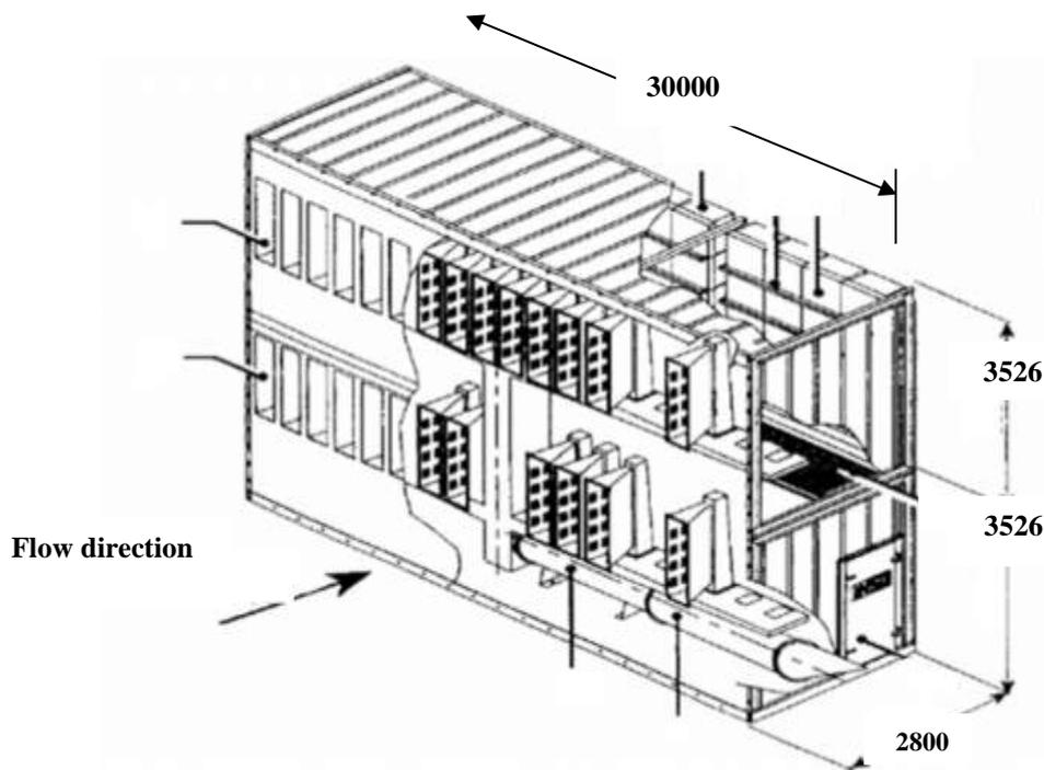
Figure 1. schematic of inertial sand separators system (dimension in mm)
