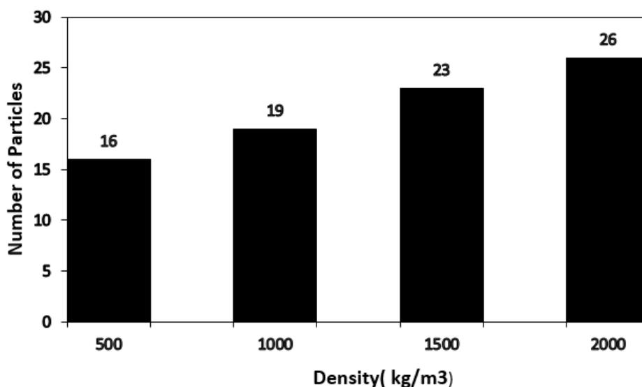
Figure 14. The total number of fan exiting particles for different densities of particles
