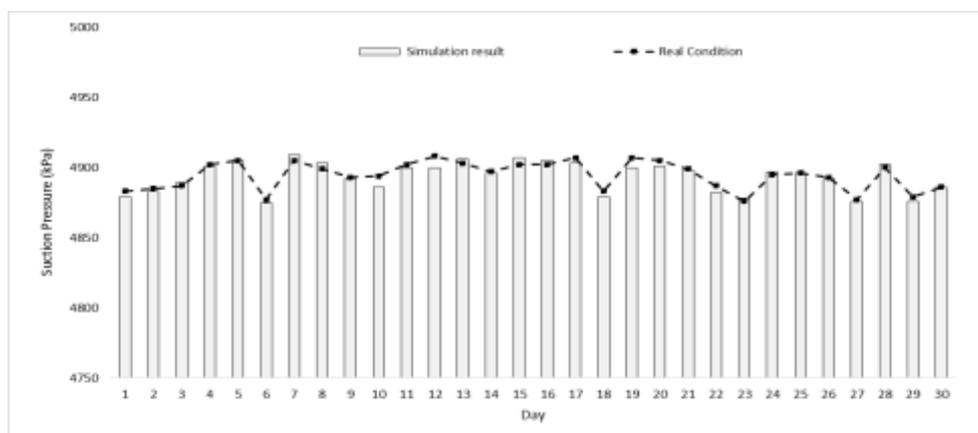
Figure 3. Comparison of real suction natural gas pressure and simulation result
