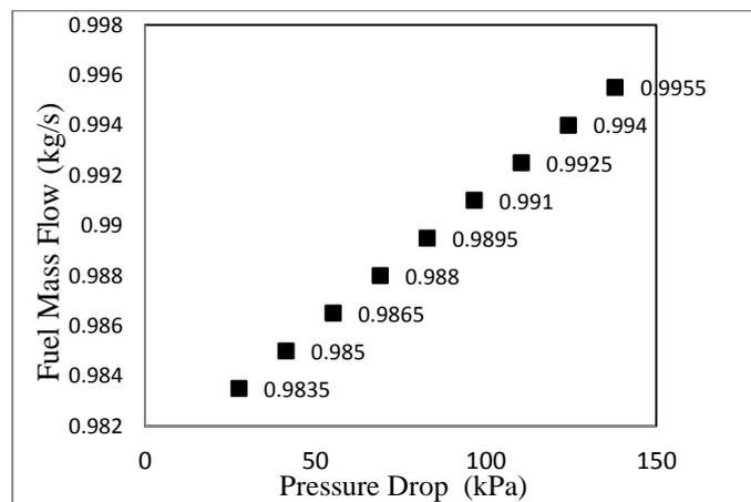
Figure 5: Analysis of pressure drop parameter and its effects on turbine fuel consumption at a natural gas compressor station
