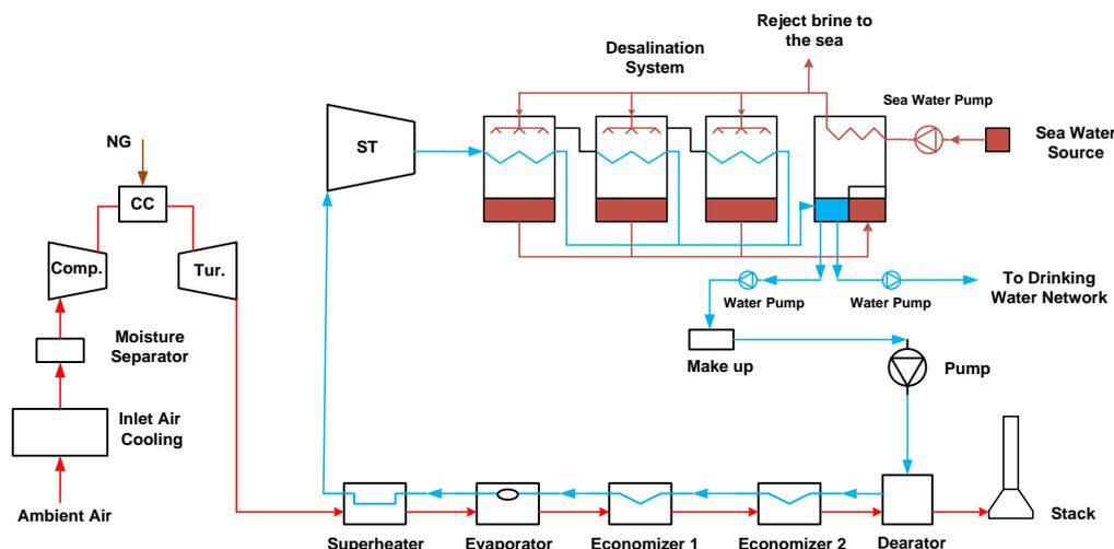
Fig. 1 The schematic diagram of the cycle of scenario 1
