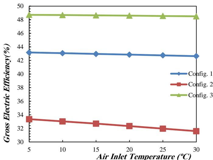
Fig. 9 Gross electrical efficiency as a function GT inlet air temperature
