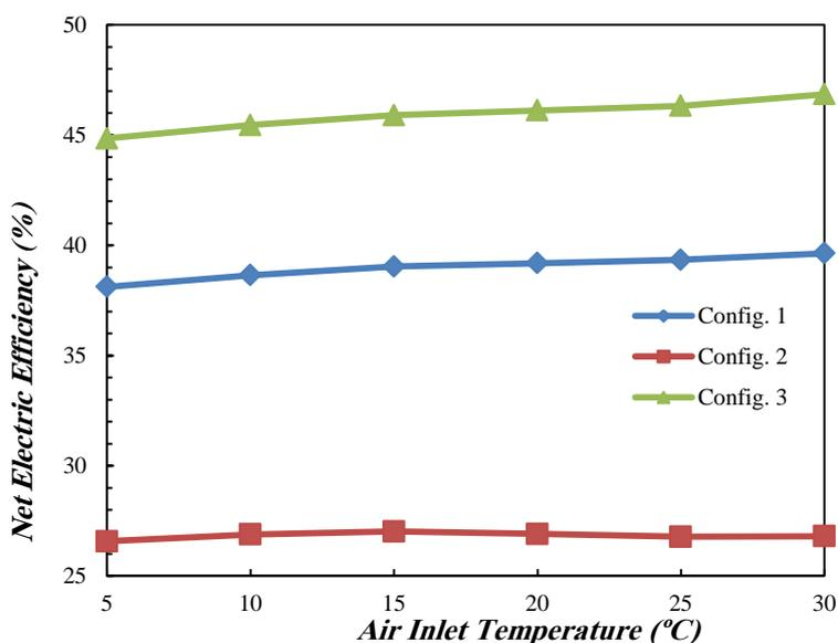
Fig. 10 Net electrical efficiency as a function GT inlet air temperature
