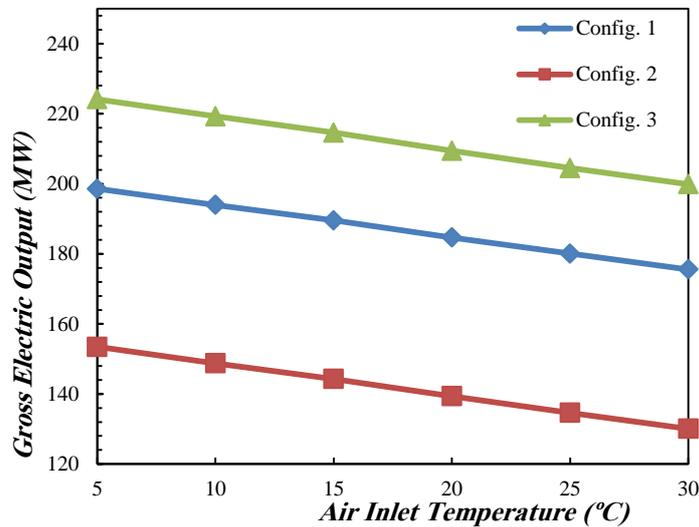
Fig. 7 Gross electric output as a function of GT inlet air temperature
