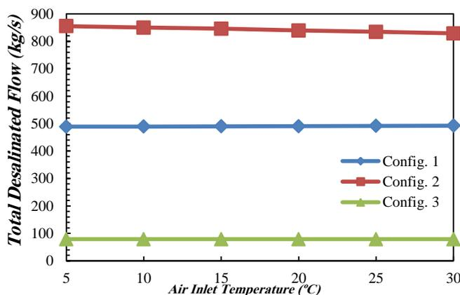
Fig. 6 Total desalinated flow as a function of GT inlet air temperature
