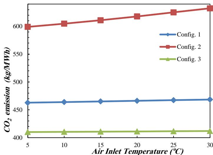
Fig. 5 Carbon Dioxide emission as a function of GT inlet air temperature
