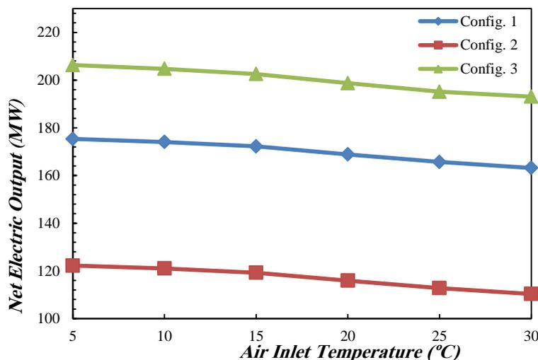
Fig. 8 Net electrical output as a function of GT inlet air temperature
