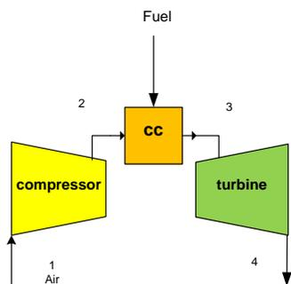
**Fig. 4 The schematic diagram of the gas turbine**
