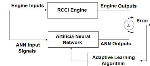
Figure 4: Direct identification of the RCCI combustion mathematical model through an ANN
