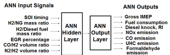
Figure 5: The used ANN active layers: a hidden layer and an output layer
