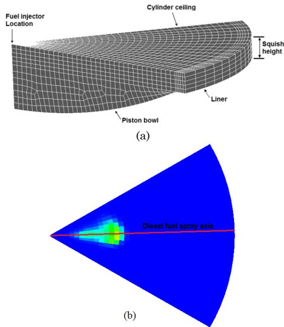
**Figure 1: (a) Three-dimensional computational grid of the selected engine (b) Diesel fuel spray axis displaying (Mabadi Rahimi, Jazayeri, & Ebrahimi, 2020)**
