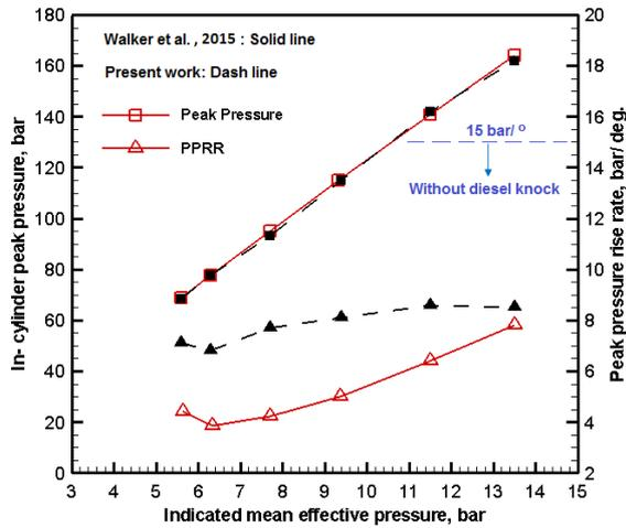
Figure 3: The engine in-cylinder peak pressure and the PPRR validation
