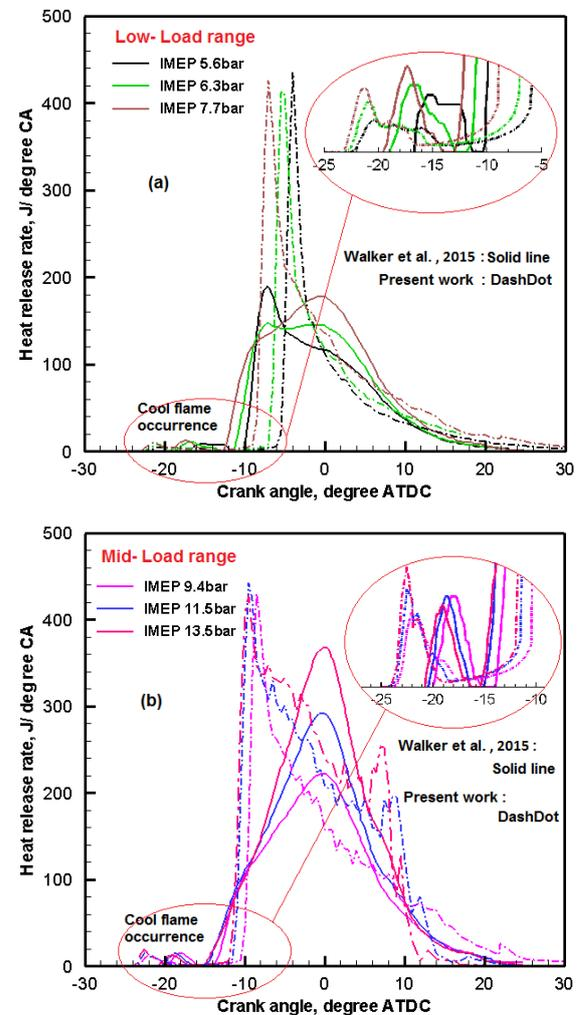
**Figure 2: The heat release rate validation for: (a) Low-Load range and (b) Mid-Load range**
