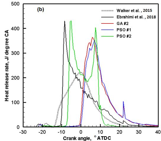
Figure 7: (a) In-cylinder pressure (b) Heat release rate for proposed items by the optimization algorithms
